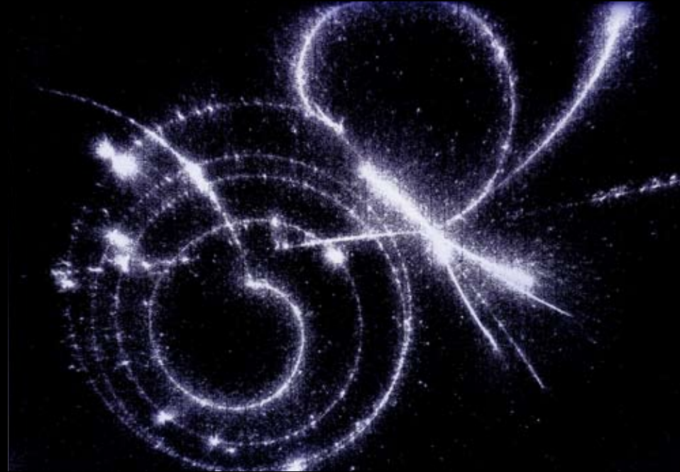
Spiraling + Muon in Bubble Chamber
