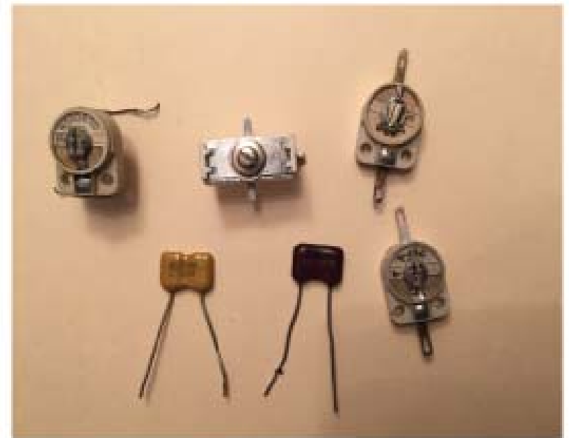
Mica fixed and variable capacitors
