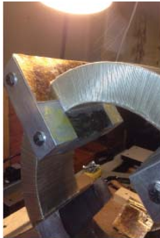
Installing cut mica plates
