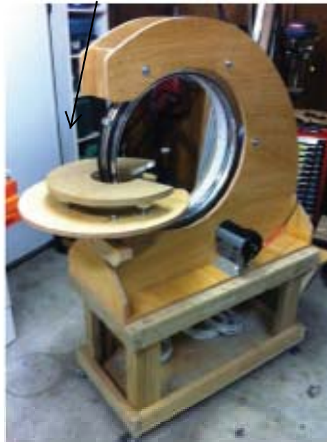
DIY Toroidal Winder
