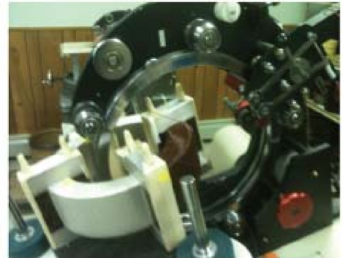
Core on winding machine
