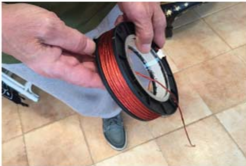
Exciter Coil with Litz wire
