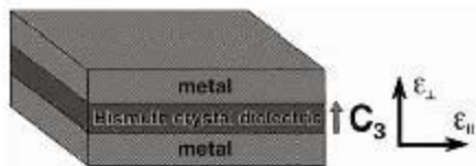
Figure 9.3. Waveguide made of monocrystalline bismuth sandwiched between two metal layers and used to demonstrate negative refraction of a 5,000-gigahertz microwave beam.
