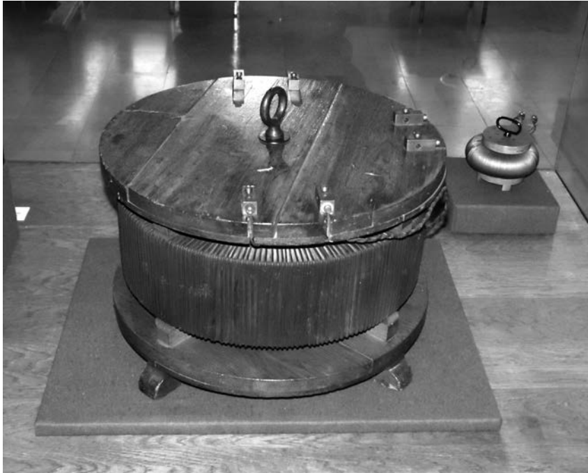
FIGURE 3.1. First transformers developed by Zipernowsky, Bláthy, and Déri in 1884-1885 in the Museum of Applied Arts, Budapest.
