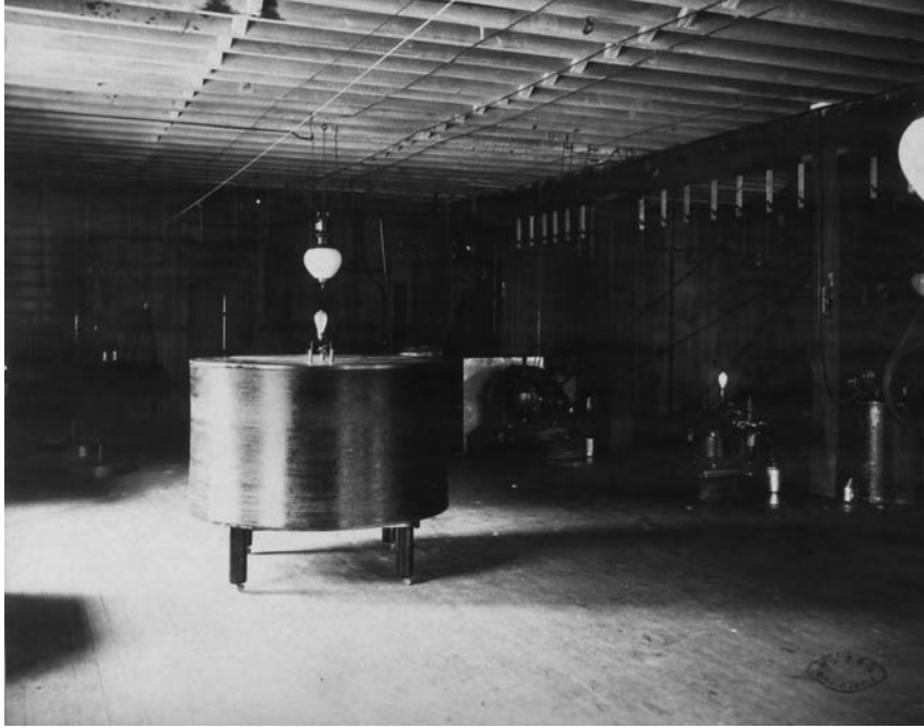
FIGURE 10.4. The receiving coil for Tesla's resonant transformer, as used in the South Fifth Avenue laboratory circa 1894.
